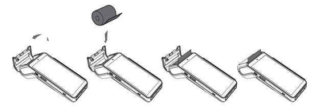
Pull the paper to the top of the terminal. Holding the free end of the paper, close the cover. Press simultaneously on both upper corners of the cover until it clips into position.
